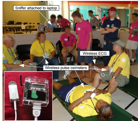
Fig. 5. The indoor treatment area of the disaster drill. Inset shows the electronic triage tag.
