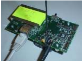
Fig. 2. Crossbow MIB600 “emote” interface board. Attached to a Mica2 or MicaZ “mote”, provides remote reprogramming and data logging capabilities.
